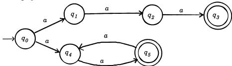
10. (a) Convert the nfa given by the following transition graph into an equivalent dfa:
