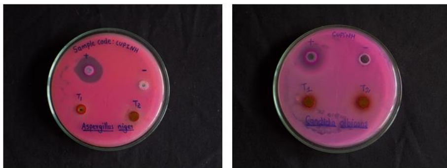
Fig.37 . Antifungal assay of Cu(II) complex of 4-[N,N-(dimethyl)amino]benzaldehyde isonicotinoylhydrazone (denoted as CUPINH) on the A. niger and C. albicans
