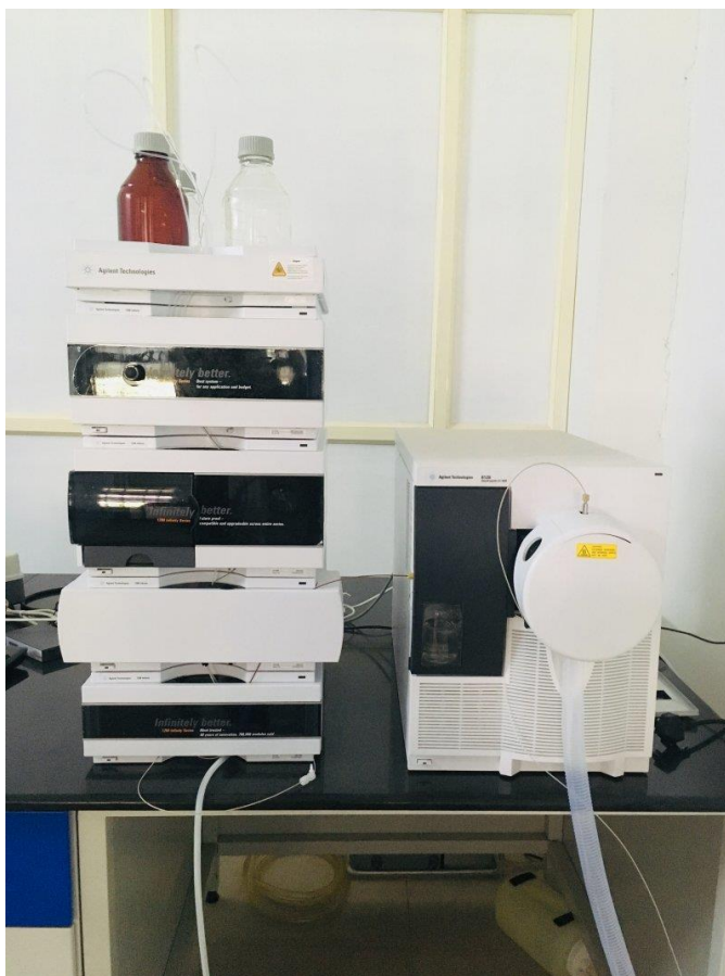
Fig.3.26. The image of High-Performance Liquid Chromatography analyser- Agilent 6100 Series Quadrupole LC / MS systems- CSIF, University of Calicut.
