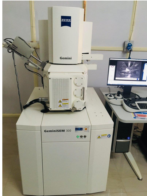
Fig. 3.13. The image of Field Emission-Scanning Electron Microscope- ZEISS GeminiSEM 300- CSIF, University of Calicut.
