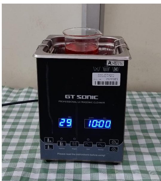
Fig.3.29. The image of GT Sonic cleaner- sonocatalytic reactor – Laboratory for Mesoscopic Science and Devices, Department of Physics, University of Calicut.
