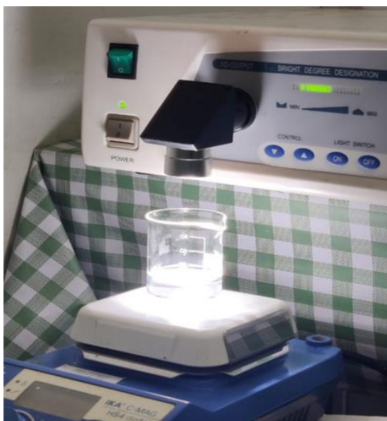
Fig.3.31. The photoreactor setup with Xe arc lamp source- Laboratory for Mesoscopic Science and Devices Department of Physics, University of Calicut.
