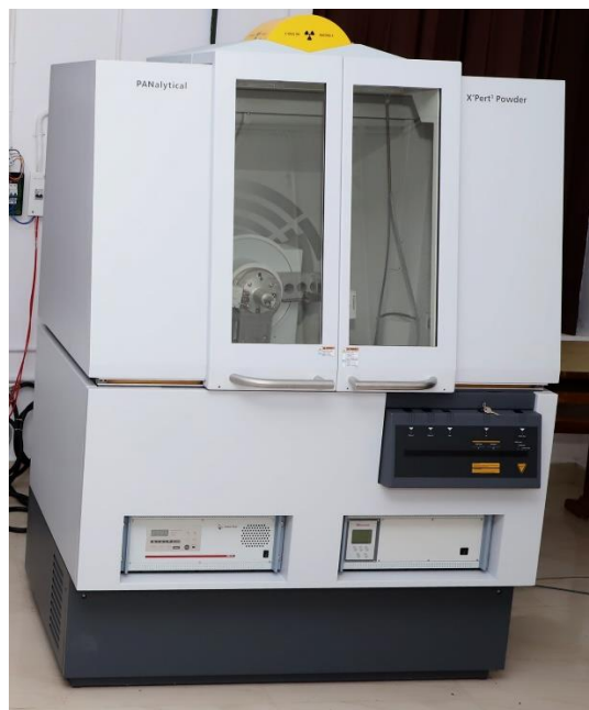
Fig.3.6. The image of X-ray diffractometer X'pert 3 Powder Multi-Purpose X-ray Diffractometer used in the study - CSIF, University of Calicut.
