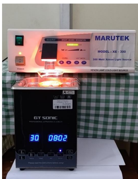
Fig.3.32. The image of sonophotocatalytic reactor-Laboratory for Mesoscopic Science and Devices, Department of Physics, University of Calicut.
