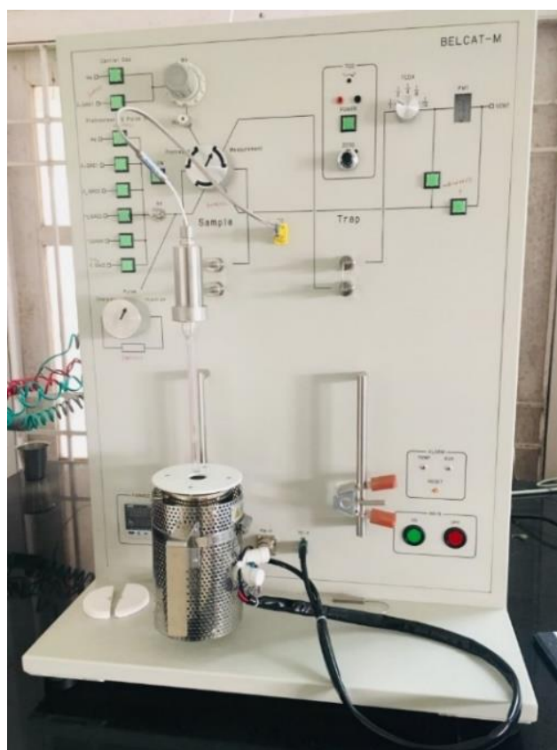
Fig.3.II. The image of Temperature Programmed Desorption (TPD) measurement system - BELCAT-M – CSIF, University of Calicut.
