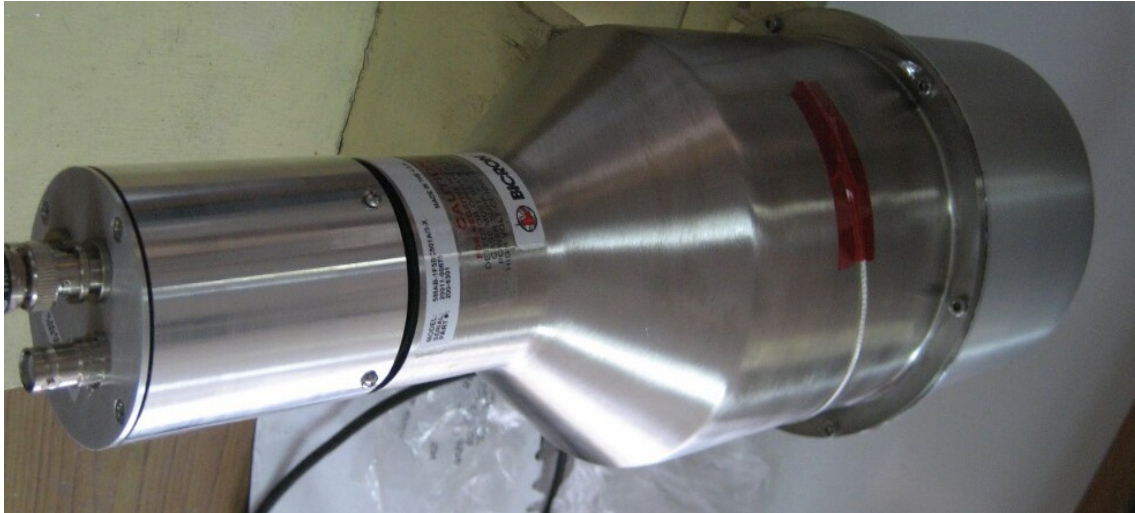
FIGURE 5.3: 5 in (diameter) x 5 in (height) BC501A liquid scintillator cell mounted on a 5 in diameter PMT
