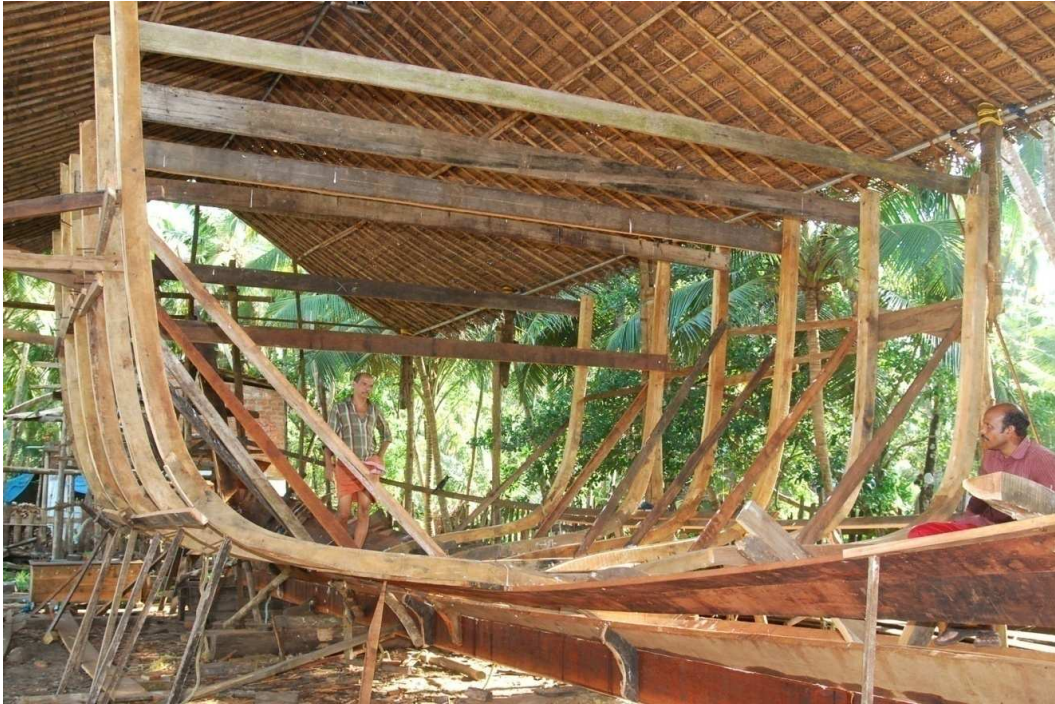
Frame Construction (Source: Photograph by Researcher)
