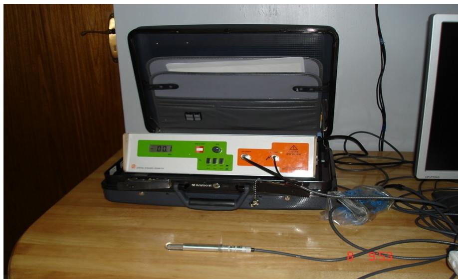
Figure 1. 5 Ionization chamber manufactured by CD high-tech, India
