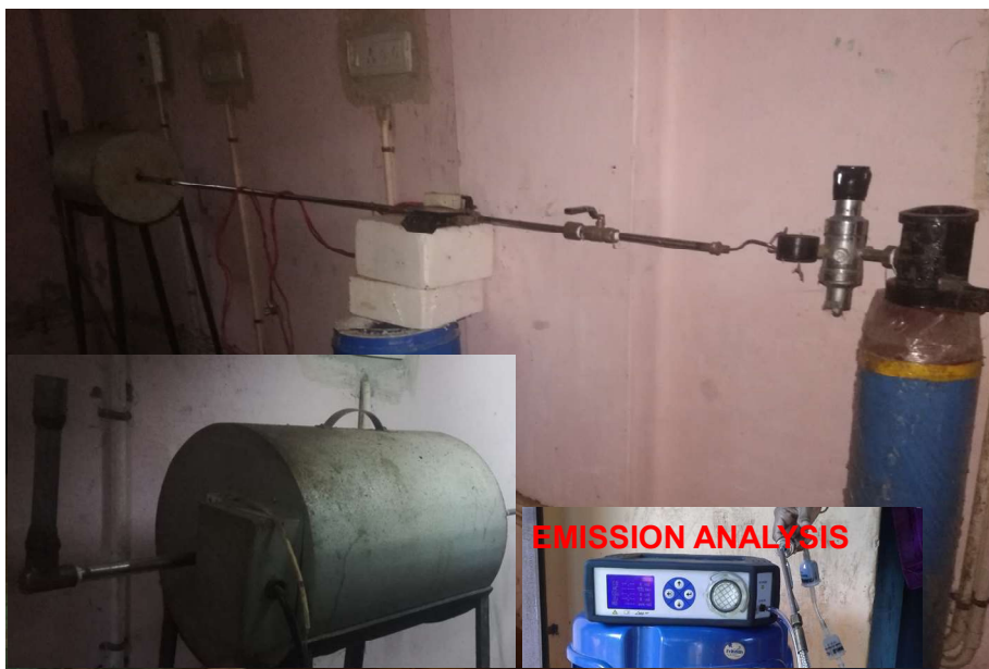
Fig. 6.2 Experimental setup for the catalytic oxidation of CO and HC.
