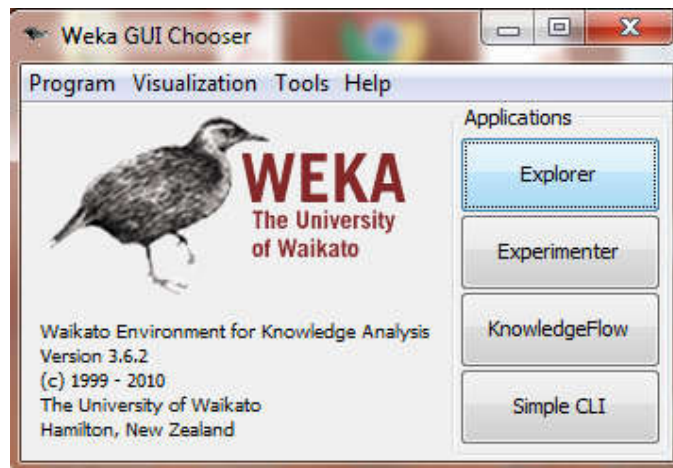
Figure 13 (a). WEKA GUI chooser is displayed with different applications involving “explorer”, “experimenter”, “knowledge flow” and “simple CLI” where various data mining tasks are performed.
