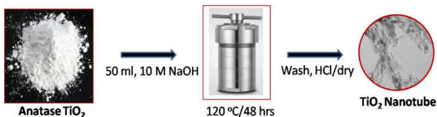
Scheme 3. 1. Schematic representation of the synthesis of TiO 2 nanotubes (TNT)
