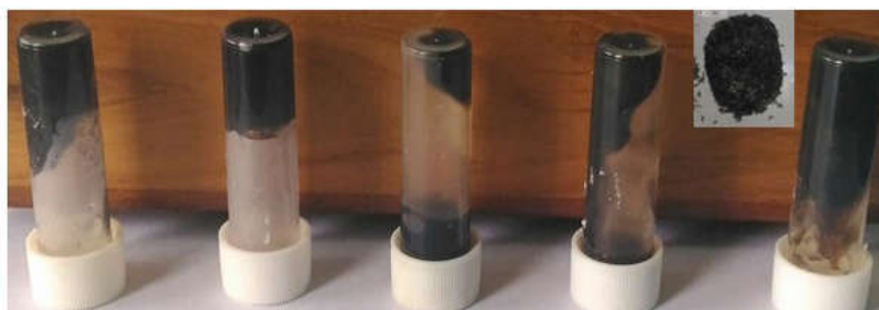
Figure 1. Digital images of Graphene Hydrogels of varying composition which can be employed as adsorbent for various pollutants. Figure in the inset presents the freeze dried images of Graphene Hydrogel.
