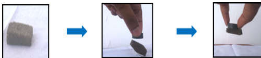
Figure 3. Manipulation of GPUF by an external magnet.
