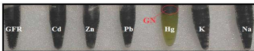
Figure 9. Impact of some environmentally relevant ions on GFU. A visual colour change from dark green to pale green is noted on addition of \text{Hg}^{2+} ions. (FLR: 1 \mu\text{M} , 10 \mu\text{L} ), GN (2 \mu\text{L} ), Metal ions (15 ppm).
