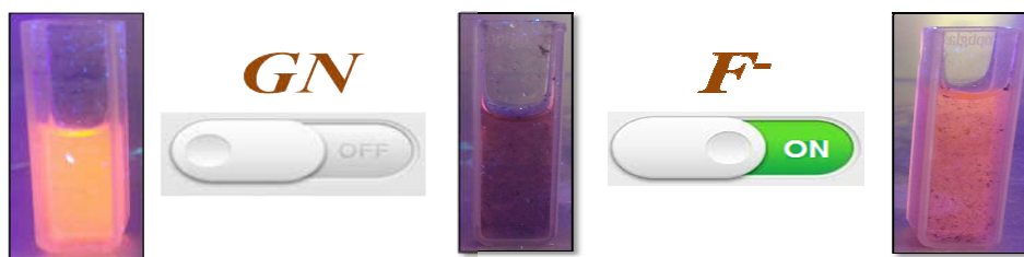
Figure 4. Colorimetric response of GRD array in presence of Fluoride ion in UV light (b) [RD-1.4mL; GN-150 \mu L; Fluoride ion-900 ppt]
