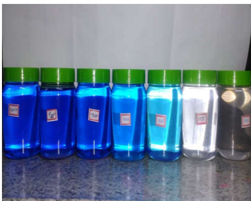
Figure 9. Dye solution evaluated for COD analysis after 35 minutes of photocatalytic degradation by Titania nanostructures
