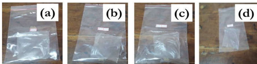
Figure 3.3 Images of (a) 5PVA film, (b) 5PVA-0.5CNC (c) 5PVA-0.75CNC and (d) 5PVA-1CNC.
