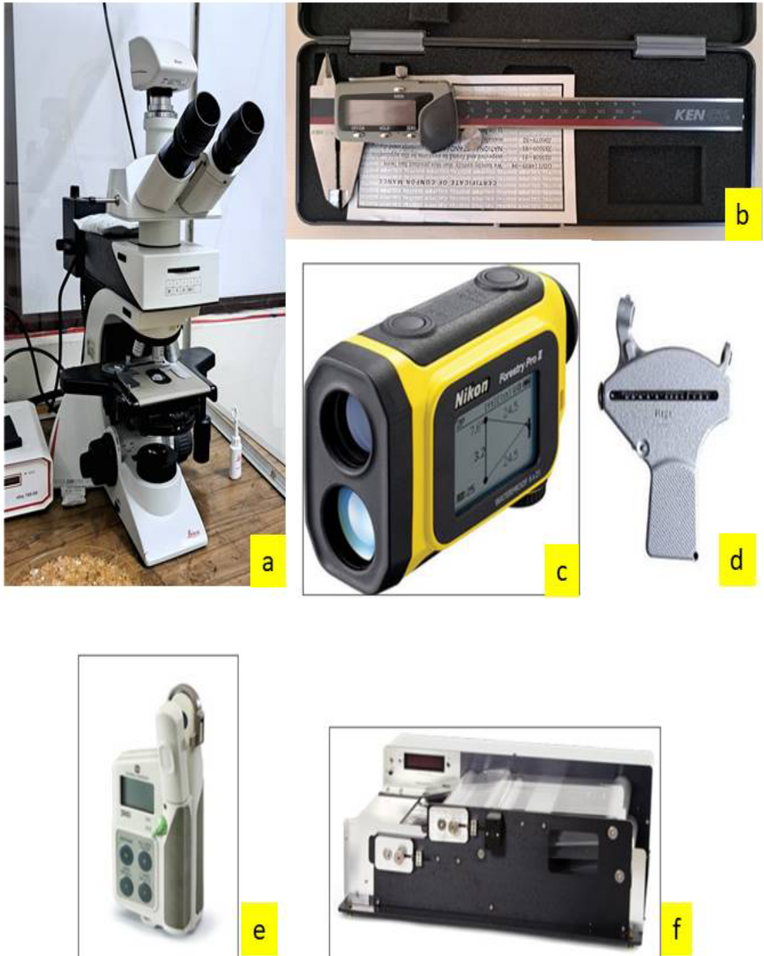
Plate 3.1. a) Image analyser (Leica Q 500 MC) , b) KEN CY 0- 150 mm digital caliper c) Hypsometer/Rangefinder, d) Haga Altimeter, e) SPAD 502 Plus Chlorophyll Meter, f) LI- 3100C Area Meter
