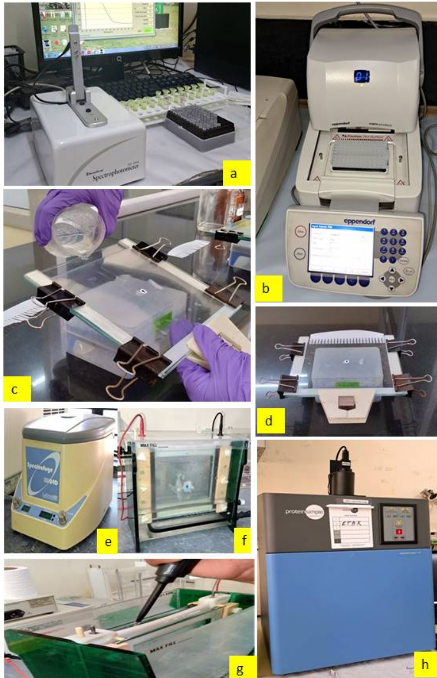
Plate 3.2. a) Spectrophotometer (Nanodrop, ND-1000), b) Gradient thermal cycler c) Preparation of acrylamide gel & pouring into the glass plates d) Glass plates fixed with the comb e) Centrifuge machine f) Electrophoresis apparatus g) Loading the DNA samples into the wells h) Gel doc system.
