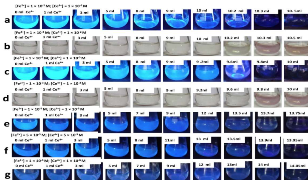
Figure 3.5. Photographs showing endpoint detection in cerimetry at different concentrations of ferrous ions using PNPA-H as a fluorescent indicator. From top row to bottom a) 1 \times 10^{-2} M in UV light b) 1 \times 10^{-2} M in visible light c) 1 \times 10^{-3} M in UV light d) 1 \times 10^{-3} M in Visible light e) 1 \times 10^{-5} M in UV light f) 5 \times 10^{-6} M in UV light and g) 1 \times 10^{-6} M in UV light.
