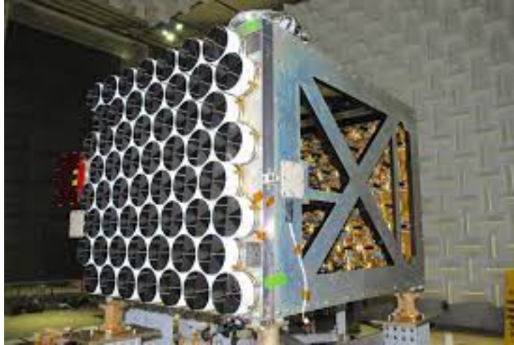
Figure 2.2: A view of NICER X-ray timing instrument without the protective blanketing. Image credit : https://www.nasa.gov/content/about-nicer
