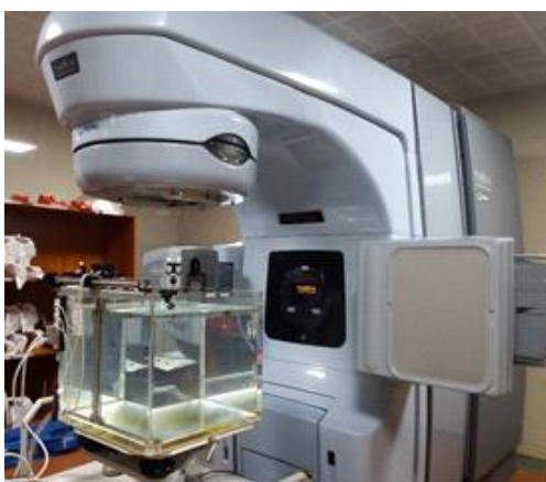
Fig 5.2 Experimental setup for the point dose measurements using radiation Field analyzer with detector
