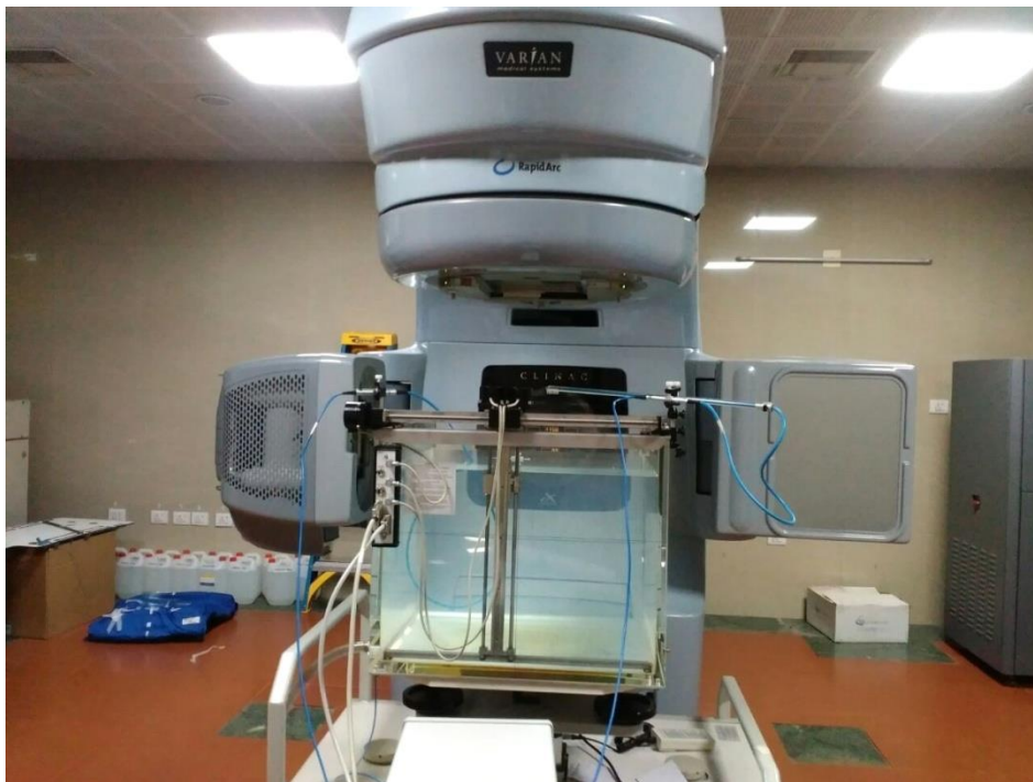
Fig 3.10 Experimental setup for the out of field dose measurements using radiation field analyzer (RFA) with semi flex ionization chamber.
