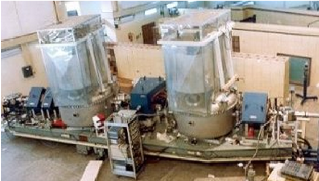
Figure 3.3: A complete view of Heavy Ion Reaction Analyzer (HIRA) setup [7], where the beam enters from the right side, it goes to the focal plane, situated on the left.
