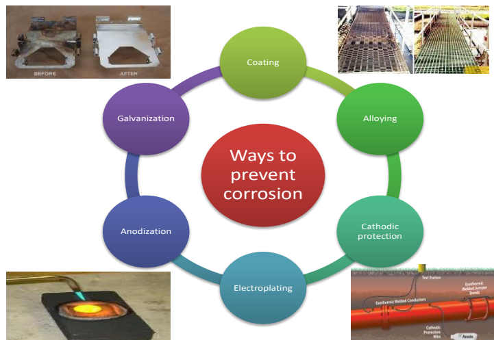
Figure 1. Pictorial representation of common methods of corrosion protection.
